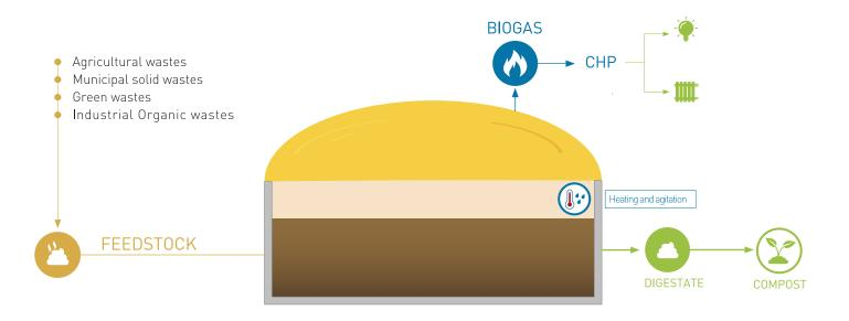
Bi'nergy® offers various standard configurations for Bi'wet®, with power outputs ranging from 18 to 300 kWe (other power options are available upon request)
