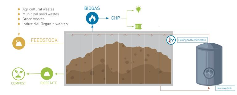
Bi'nergy® offers various standard configurations for Bi'dry®, ranging from 2 to 15 digesters, with power outputs varying from 18 to 300 kWe (other power options are available upon request).
